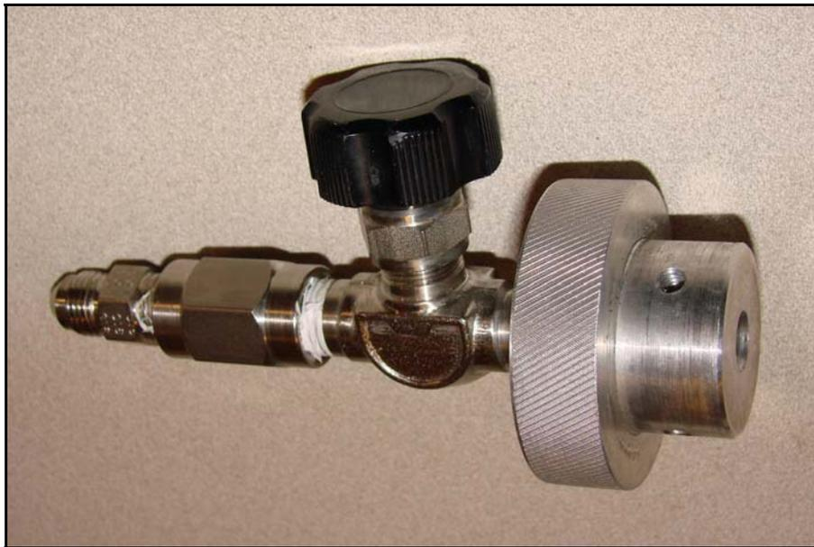
The picture above shows from left to right the hose adapter, coupling, needle valve, and the orifice body. The wand and braided hose have been removed.
