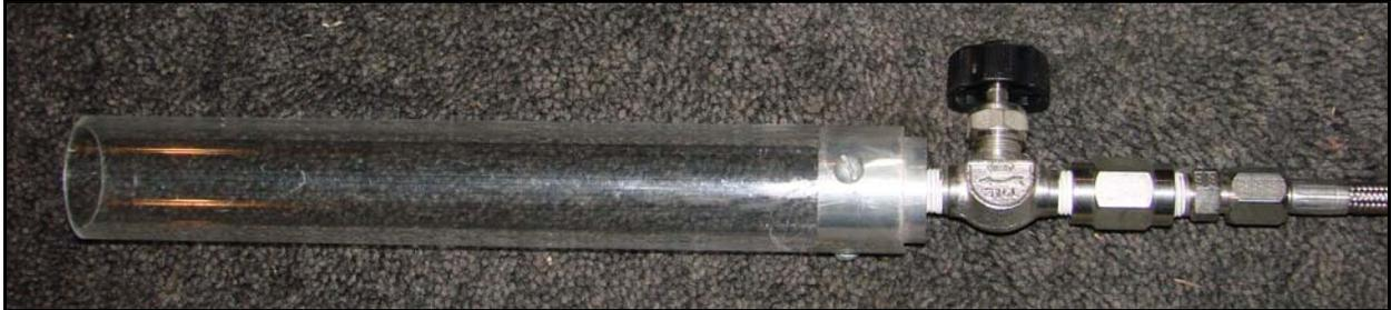
Above is the short wand model. Over time we still got small cracks around the screw holes. When you drill the attachment holes in the wand make them larger than needed to allow for expansion and contraction and leave the screws a little loose.
