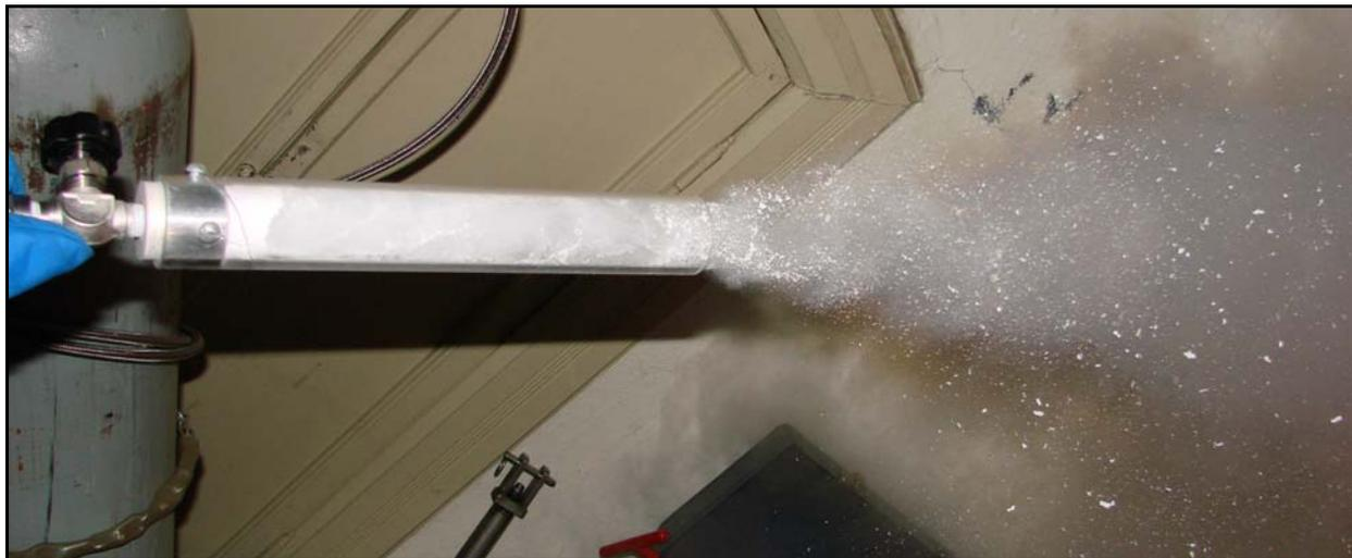
This picture shows the CO<sub>2</sub> snow apparatus in operation. Note the flakes of snow in the right of the picture.
