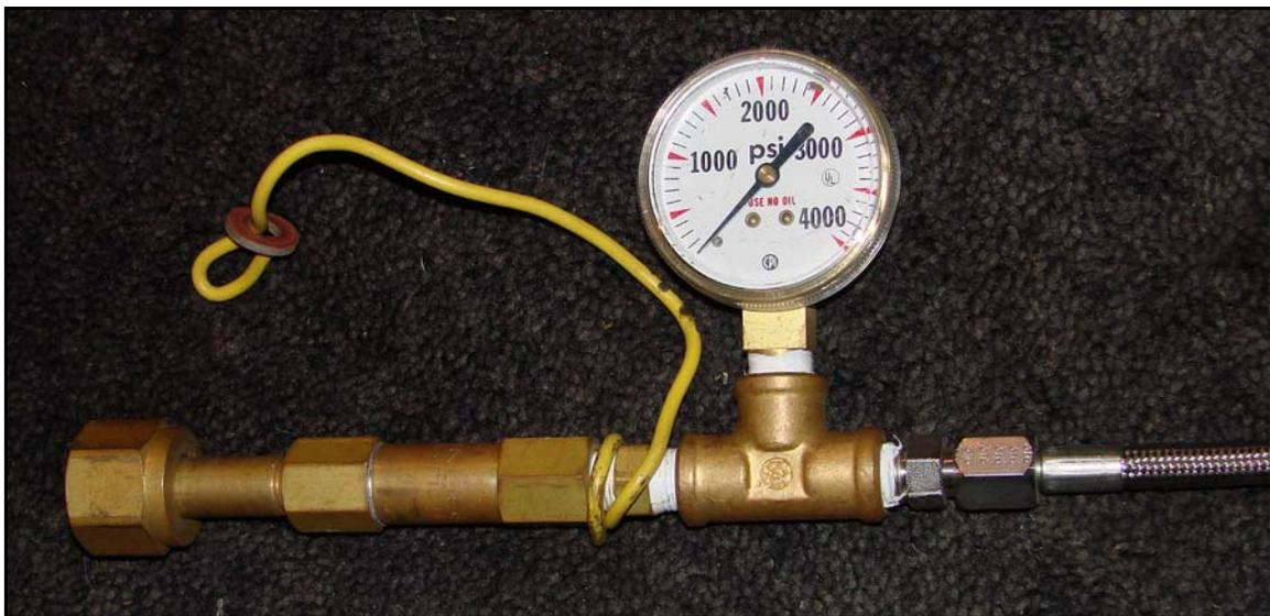
This is our first model with inline filter, pressure gauge, and brass fittings. The gauge is not necessary and this particular gauge is rated for much higher pressures than needed. Pressure in a Co<sub>2</sub> cylinder is a little over 600 psi.
